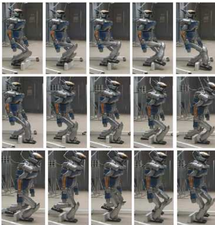
Figure 3.47: Quasi-static stepping over performed by Guan [5]
