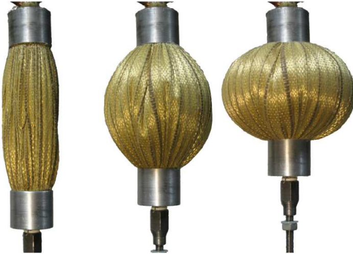
Figure 2.1: Photograph of 3 contraction levels of the 1 st generation of PPAM
