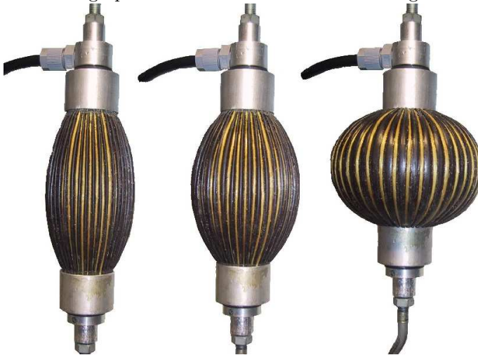
Figure 2.2: Photograph of 3 contraction levels of the 2 nd generation of PPAM
