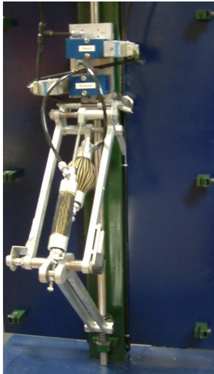
Fig.1.6: ADAM, 1DOF hopping robot with PPAM
