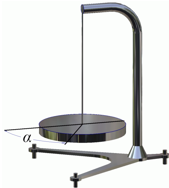
Fig.2.9: Didactic torsion pendulum setup.
