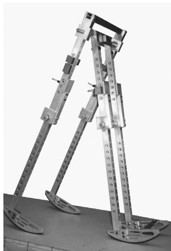
Fig.2.6: Close copy of McGeer's walker by Garcia [2.29]
