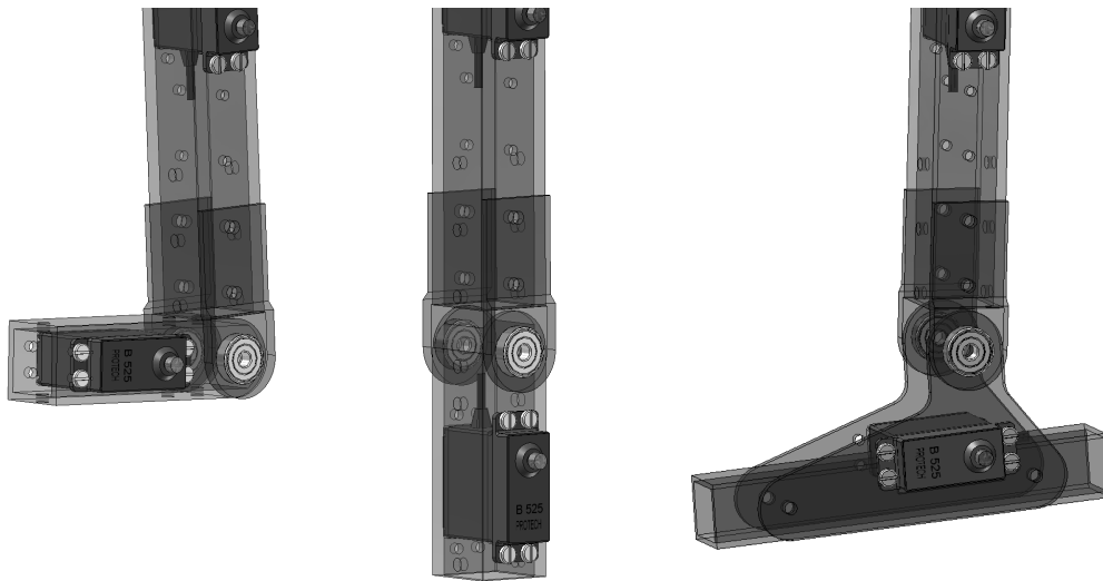
Fig.5.3 Placement of servomotor in foot
