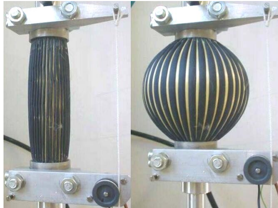
Fig 1 Photograph of the deflated and inflated state of the PPAM
