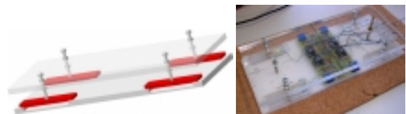
Fig. 3 - Sensitive foot base. Model and real device.
