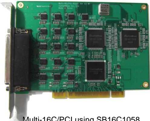
Multi-16C/PCI using SB16C1058 with 256-byte FIFO
