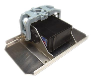
4. Attach the joints of upper arm, bottom arm and arm base by 2.6-8 tapping screws. (1 for each)
