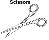
It is used for cutting the cowl, decal and the sponge. To cut the cowl (made of polycarbonate), strong scissors are suitable.
