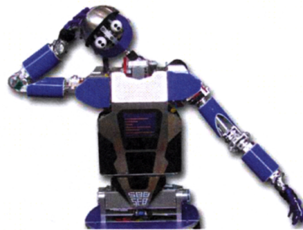
Fig. 1 Upper body of the humanoid robot ARMAR III
