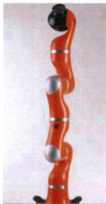
Fig. 3 The DLR/Kuka lightweight robot arm [3]
