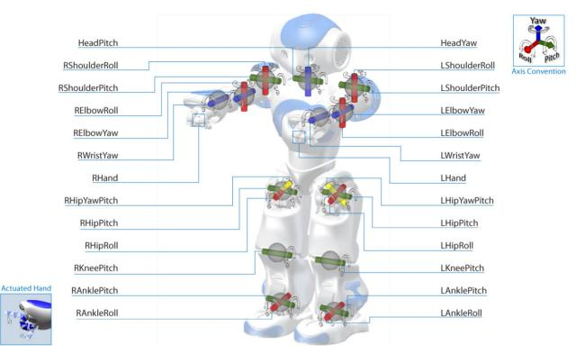
The scheme above presents all the robot's axes. Together, these axes allow 25 degrees of freedom, which when coupled with the inertial sensor, the force sensitive resistors, the Hall effect sensors, the infrared receiver and the sonar sensors, allows Nao® a high level of stability and fluidity in its movements.
