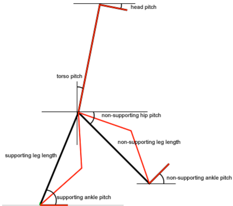
Figure 4.5: Simplified pitch parameters, relative to the ground plane (supporting foot), replacing the knee joint with a linear ‘virtual leg’:
