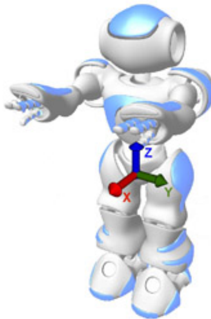
Figure 2.3: Axes of Nao's IMU
