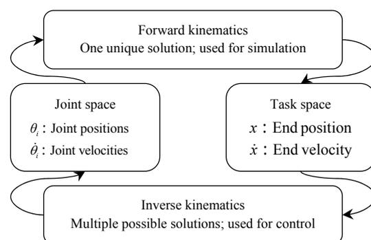
Fig. 1 Comparison of forward and inverse kinematics
