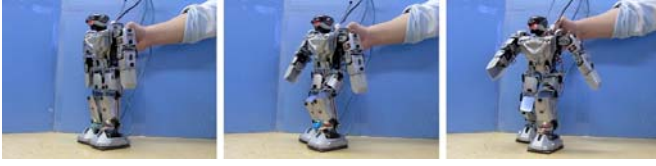
Fig. 16. Actual movement when human pushing back on right side
