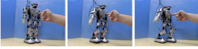
Fig. 15. Actual movement when human pushing front on left side
