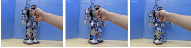
Fig. 14. Actual movement when human pushing front on right side
