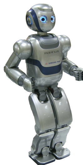
Fig. 1. Biped humanoid robot Mahru III.
