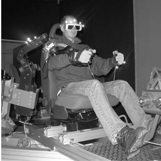
Figure 2 The PERCRO Laboratory (Scuola Superiore di studi Universitari S. Anna, Pisa, Italy) has extensive experience with the development of exoskeleton-type haptic interfaces
