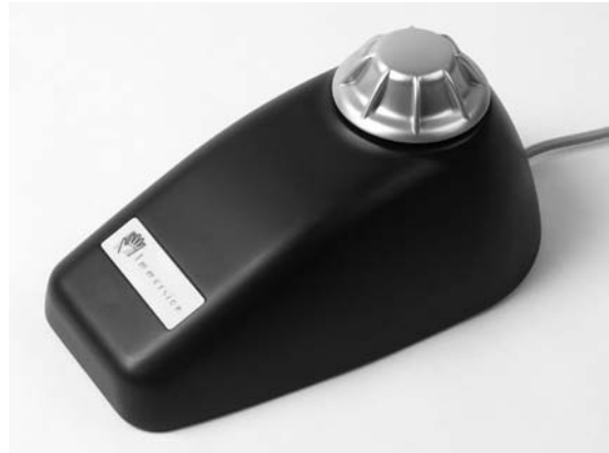
Figure 5 From Immersion Corp. a one degree of freedom device for navigation in user interfaces
