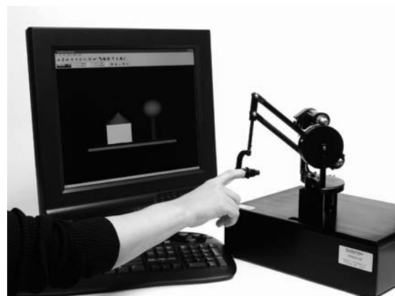
Figure 3 SensAble Technologies Inc. three degree of freedom Phantom™ 1.0, a common device for general research
