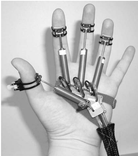
Figure 6 From the Human-Machine Interface Laboratory of Rutgers University, the Master II-ND virtual reality force-feedback glove (new design)
