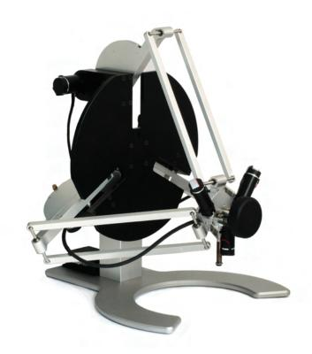
The **delta.6** is a high performance force feedback interface based on the delta manipulator. It offers 6 active degrees-of-freedom in translation and rotation and offers a **larger workspace** than omega.x devices. Thanks to its unique parallel mechanical design, the **delta.6** can convey **large continuous forces and torques** anywhere in its workspace.
