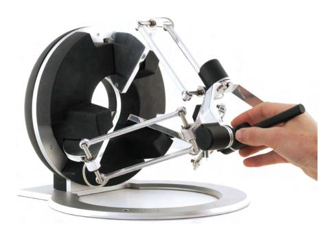
The omega.6 is the most advanced pen-shaped force-feedback device available. Building on the omega.3 base, its design provides perfect decoupling of translations and rotations. The combination of full gravity compensation and driftless calibration contributes to greater user comfort and accuracy. Conceived and manufactured in Switzerland, the omega.6 is designed for demanding applications where performance and reliability are critical.
