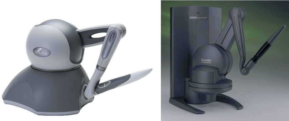
Figure 1.4: The Sensible PHANToM OMNI (left) and PHANToM Desktop (right) haptic impedance-based desktop devices [20; 19].
