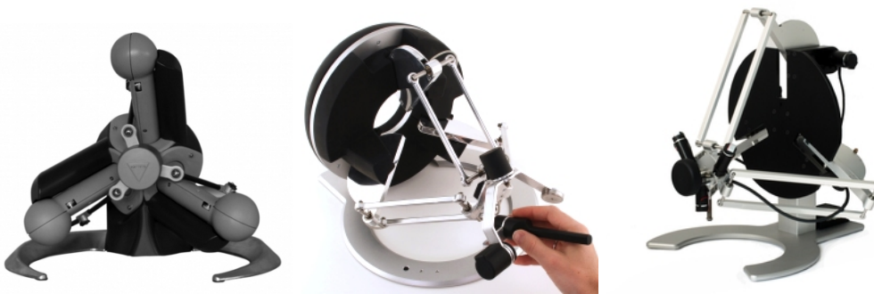
Figure 1.5: The Haption Virtuoso 6D Desktop (left) , the Force Dimension Omega (middle) and Delta (right) haptic impedance-based desktop devices [21; 22; 23].
