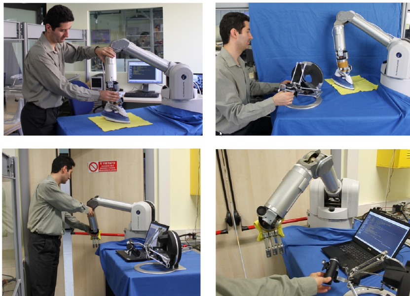
Figure 1.13: Retrieving position and force profiles from different tasks, such as ironing a piece of cloth or opening a door, for teaching purposes [4].
