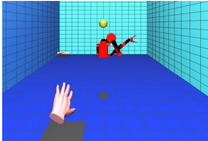
Figure 1.15: Virtual environment used for learning by demonstration with a serial arm catching a ball in mid-air [36].
