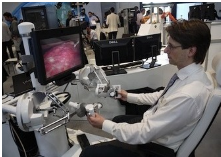
Figure 1.9: The Force Dimension Sigma haptic device in a medical application [29].
