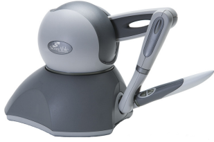
Fig. 5 - The haptic device is an OMNI model with 3-DOF force feedback.
