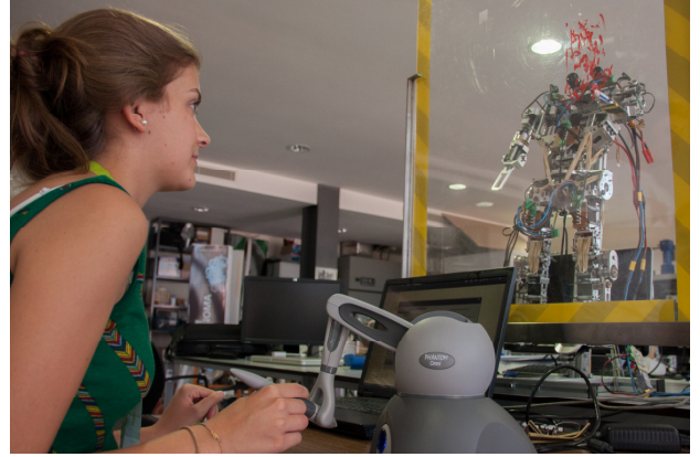
Fig. 6 - Teleoperation of the robot arm with force feedback.
