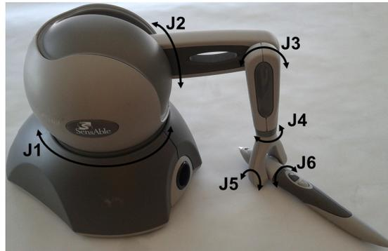
Figure 2.4: Phantom Omni DOF's.
