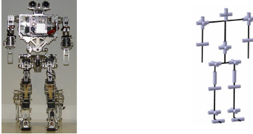
Figure 2.1: Physical humanoid robot (left) and distribution of DOF by the full-body structure (right) [6].
