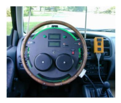
Figure 1.7: ATI/Heitz Sprint 3 steering controller
