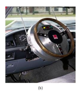
Figure 1.6: SEA, Ltd. Automated Steering Controller system
