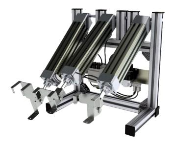
Figure 3.1: Pedal actuator unit
