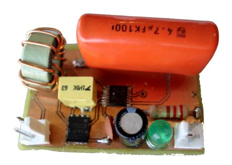
Figure 2.5: Power supply for the sensors network
