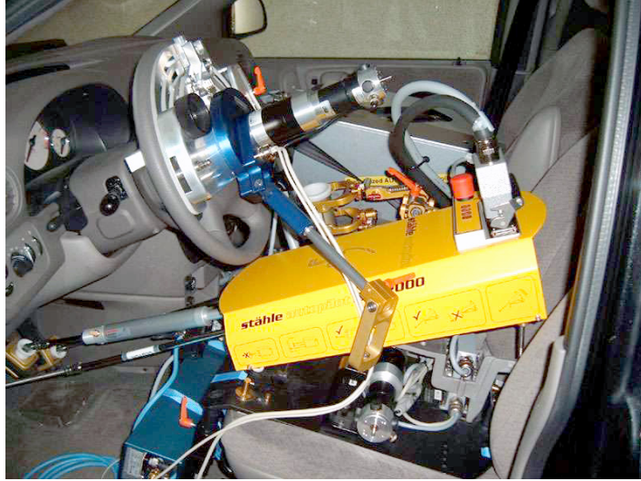
Figure 1.8: Stähle SPF2000FF robot driver
