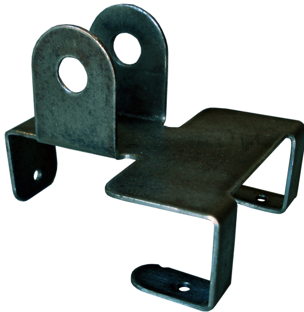
Figure 3.6: Clutch and brake pedals attachment
