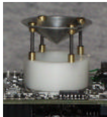
Figure 4: The localization sensor with acoustic reflector.
