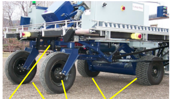
Rocker-Boogie Arm-axle with dual offset casters Differential Drive Tube DC Motor & manual hub
