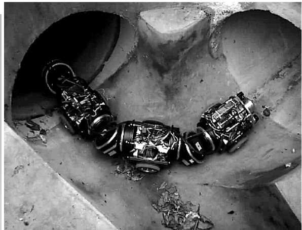
(b) Sewer robot prototype MAKRO 1.0 performing a turn in a dry sewer.
