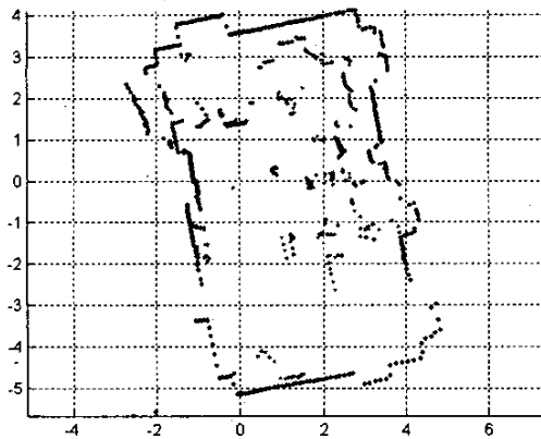
Figure 4. Virtual 2D scan (black), Regular 2D scan (50cm height, red)
