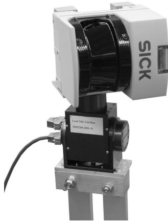
Fig. 1. 3D scanner (yawing scan) consisting of a 2D laser range sensor (Sick) and a servo drive (Powercube)
