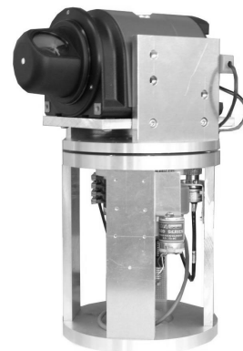
Fig. 9. Scan drive prototype with IBEO 2D range finder
