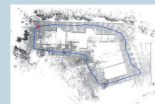
the corresponding closed-loop 3D map seen from above, generated online from dozens of individual 3D scans
