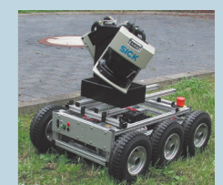
Automatic 3D map building with the mobile robot VolksBot and the 3DLS-K
