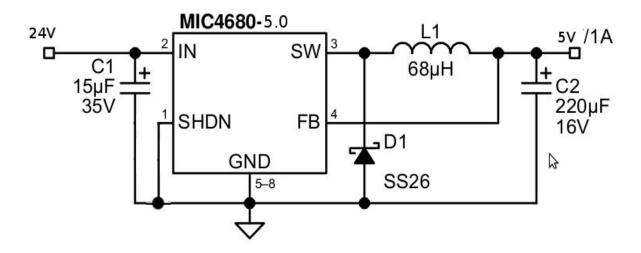
To make the winding, a toroid nucleus was used and tested with an OPAMP oscillator but best option is to buy one. The capacitors are recommended to be solid tantalum, careful that prices vary a lot depending on maker and supplier. The circuit can fit into roughly the same space of the 7805.
