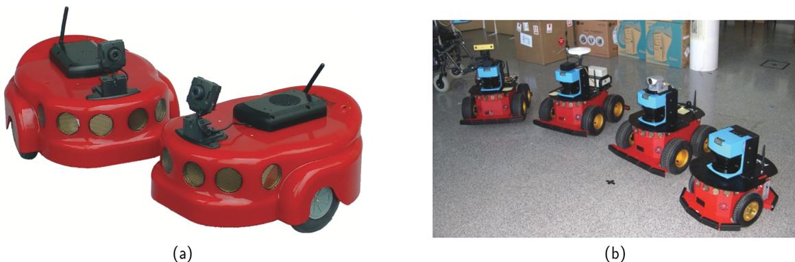
Figura 1.8: (a) Robô AmigoBot<sup>™</sup> da Mobile Robots<sub>INC</sub>; (b) Robôs Pioneer 3-AT e 3-DX da Mobile Robots<sub>INC</sub>.
