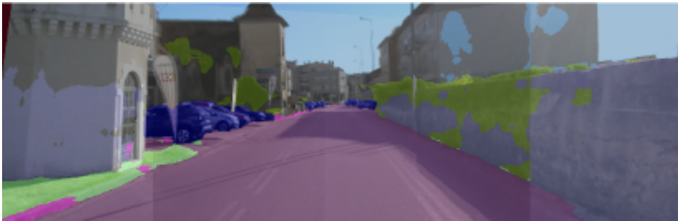
Figure 5.10: Segmented panoramic image with argmax .
