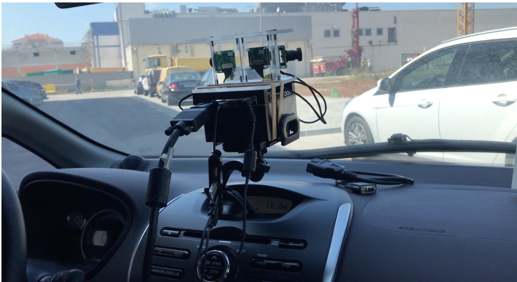
Figure 4.7: Jetson AGX Xavier and cameras setup in AT-LASCAR2. A suction stand was used to hold the Jetson AGX Xavier setup with the cameras. This was placed on the dashboard of the car and a small sponge was used on the top to prevent movement during the images acquisition.
