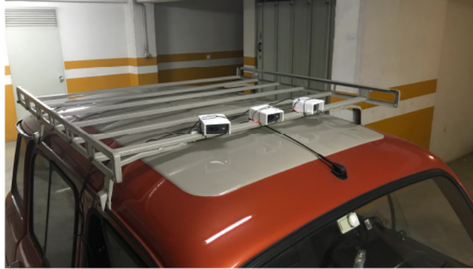
Figure 5.3: Positioning of cameras for data gathering.
