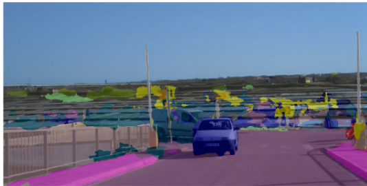
(c) Segmented image with ContextNet 2x model trained on CityScapes
