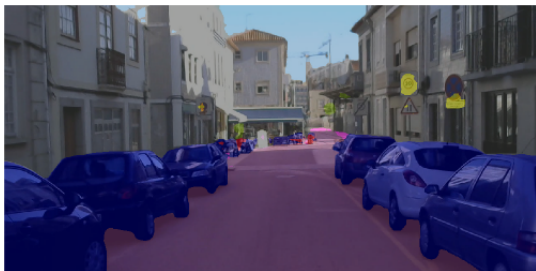
(a) Well segmented road
