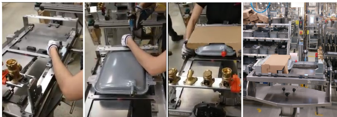
Fig. 1: Example of a real workstation where the structure of a gas boiler for water heating is manually assembled. The collaborative robot may assist the assembly task by placing the parts in the jig, while coordinating its actions with those of the human who is focused on the riveting process.
