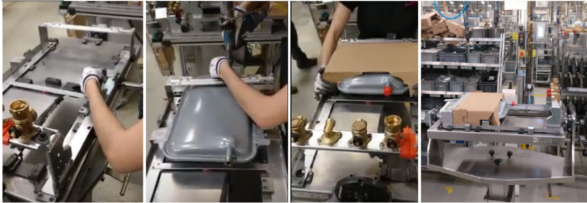
Figure 1.2: Different views of the current workstation used for the manual assemblage of the structure of a gas boiler for water heating.
