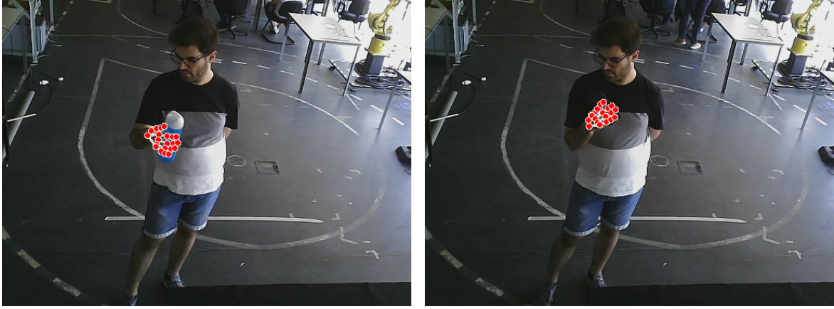
Figure 4.5: Points detected on the pictures in Figure 4.4 by Mediapipe Hands Model.
