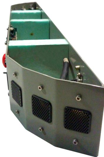
Figure H.8: Intervention performed to add resistance on the rear zone.
