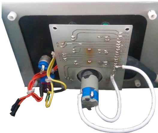
Figure H.6: PCB board for the status panel.
