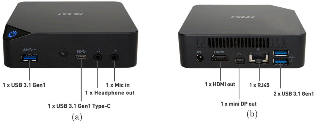
Figure 3.7: Mini PC MSI Cubi 2, front view (a) and rear view (b). Adapted from [38].
