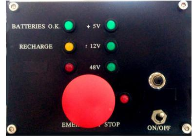
Figure 4.15: LED status panel on Robuter’s back. Check description on Table 4.3.
