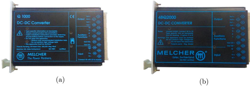
Figure 3.4: DC/DC converters Q1000 (a) and 24Q2000 (b).
