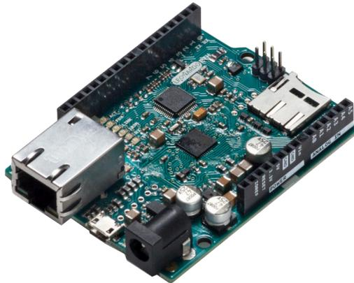
Figure 3.8: Arduino Leonardo Ethernet. Adapted from [39].
