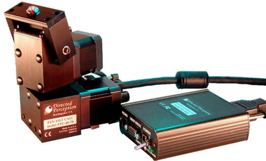
Figure 3.11: Pan-Tilt Unit FLIR PTU-D46-17. Adapted from [42].
