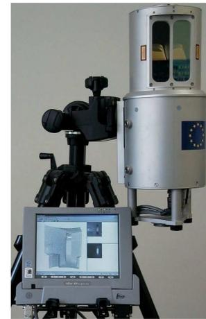
**Figure 2: Laser range scanner.**
