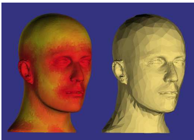
Figure 4. The sampling spacing required to correctly reconstruct a surface is proportional to the distance to the medial axis. On the left is a surface reconstructed from a dense sample. The color represents estimated distance to medial axis—red means close. On the right, we use the estimated distance to thin the data to a .5-sample (meaning that the distance to the nearest sample for any point on the surface is at most half the distance to the medial axis), and then reconstruct. There were about 12K samples on the left and about 3K on the right.
