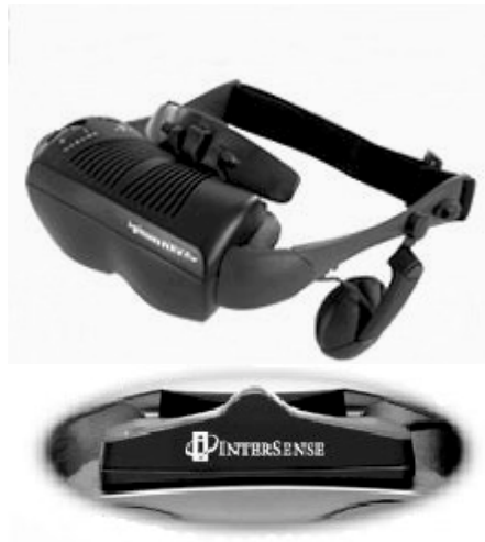
Fig. 16: (a) Head Mounted Display and (b) 3DOF Sensor for future Virtual Reality applications
