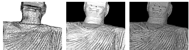
Figure 6: A closed view of a 3D model of the Bamiyan Buddha represented in wireframe, flat shaded and textured mode [Gruen et al., 2002c].
