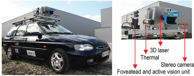
Fig. 1 – The car with external sensors shown.
