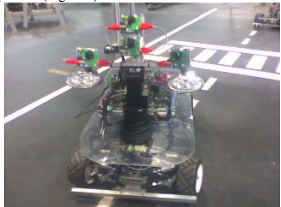
Figure 2 – Atlas MV Robot with the multi-camera perception unit
