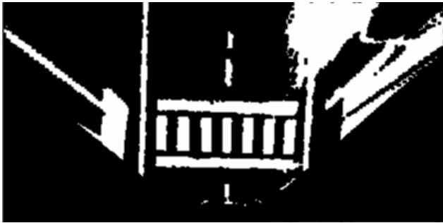
Figure 13 - Sparse Output_{img} after threshold, and morphological closing.
