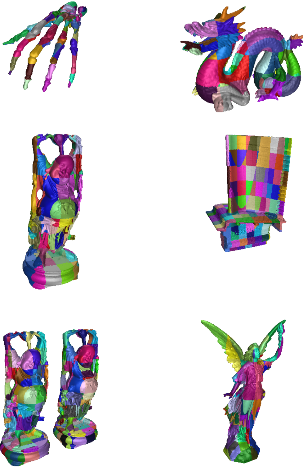
Figure 4: Reconstructed surfaces from SKELHAND (327,323 points), DRAGON (437,645 points), HAPPY (543,652 points), BLADE (882,954 points), DOUBLEHAPPY (1,087,304 points) and LUCY25 (3,505,407 points). Surface patches from different boxes are shown with different colors; see the color plate.
