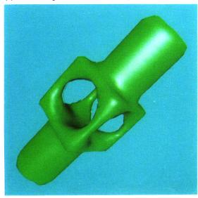
(f) Final surface after edge collapses Figure 2: Reconstruction of ray-traced CSG object (continued).
