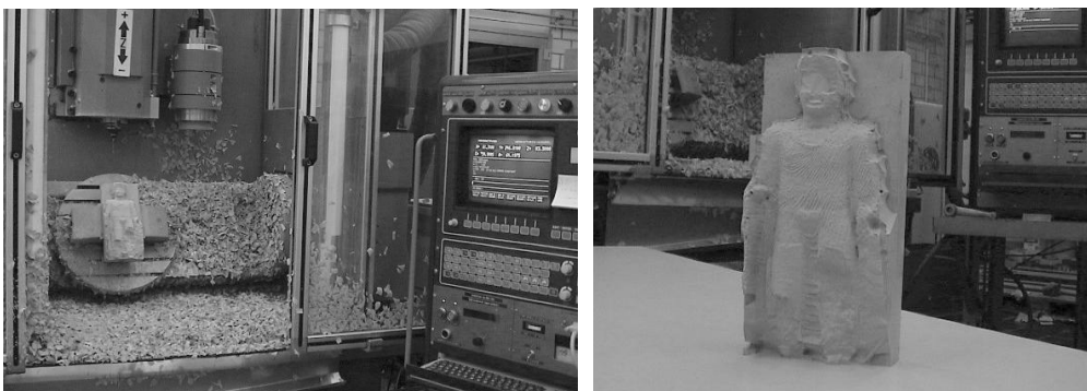
Figure 10: The milling machine used for the model carving at work (left). The resulting statue of the Great Buddha of Bamiyan at scale 1:200 (right)
