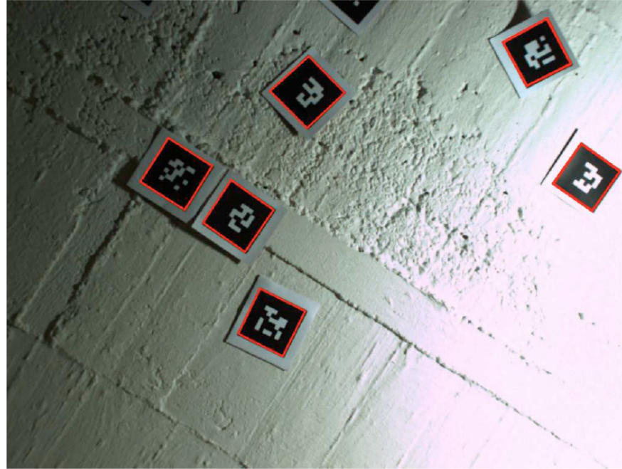
View of the robot: detected visual landmarks on the ceiling
