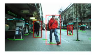
Figure 1: Example result on the Bahnhof sequence. Green line indicates the stixels bottom, blue line the stixels top and the red boxes are the obtained detections.
