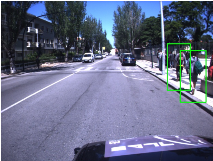
Figure 4.9: Example result 2 - In bright environments, close range pedestrians walking on the sidewalk are usually detected.
