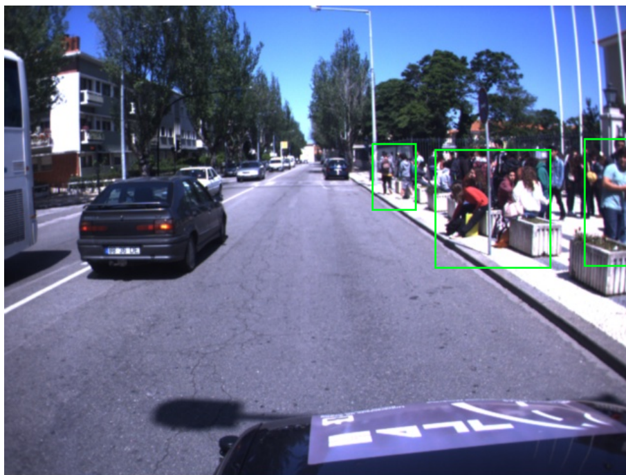
Figure 4.4: Ground truth example 3 - Groups of pedestrians standing close to each other are assumed to be only one target.
