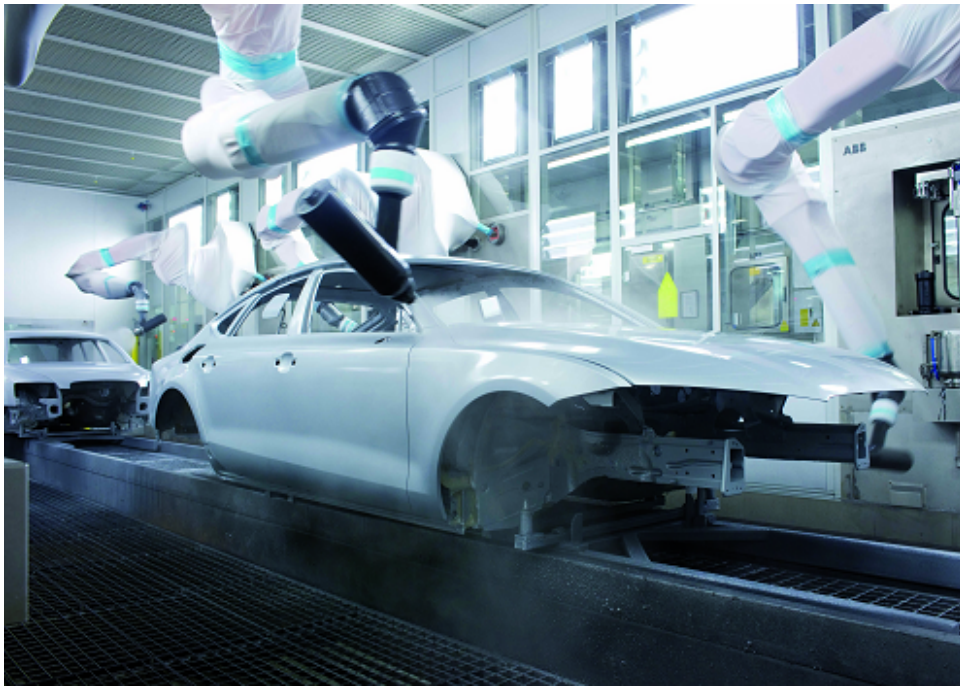
Figure 1.2: Audi's car painting production line.
