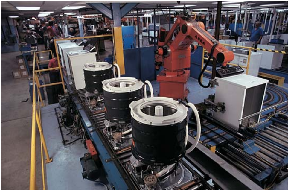
Figure 1.3: Speed Queen company assembly line.
