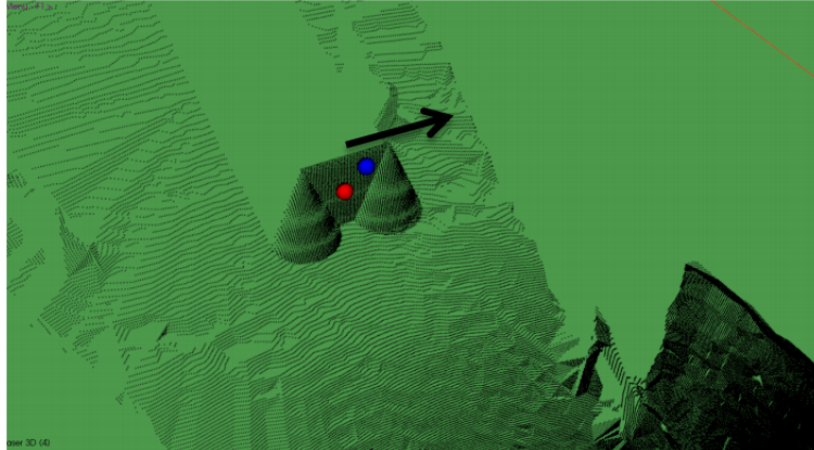
Figure 1.9: Calibration object detection in 3D data. [12]
