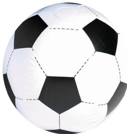
Figure 3.5: Real ball used as calibration target. The diameter is 107cm.
