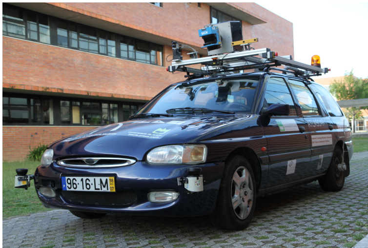
Figure 1.2: The ATLASCAR and some of its sensors.
