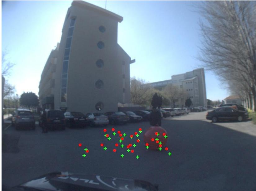
Figure 5.12: Randomly acquired ball centers by the camera in its image plane (green + symbol) and projected ball centers from Sick LMS151(A) (red dots).
