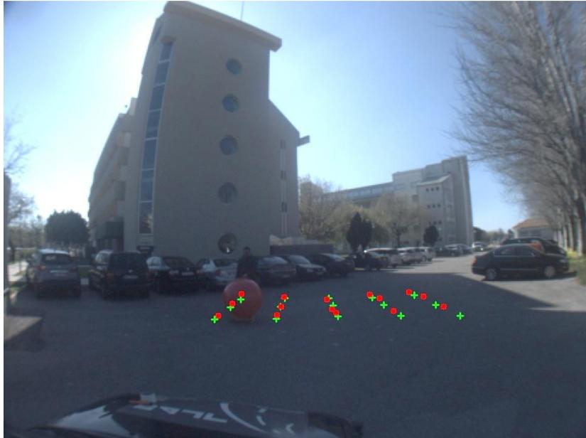
Figure 5.8: Grid pattern ball centers detected by the camera in its image plane (green + symbol) and projected ball centers from SICK LMS151(A) (red dots).
