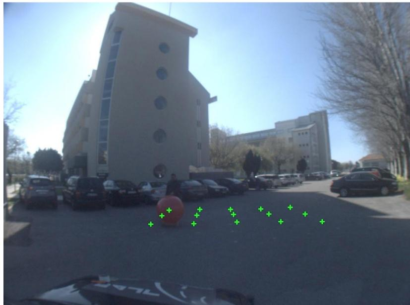
(b) Ball centers to be used with the extrinsic camera calibration method.
