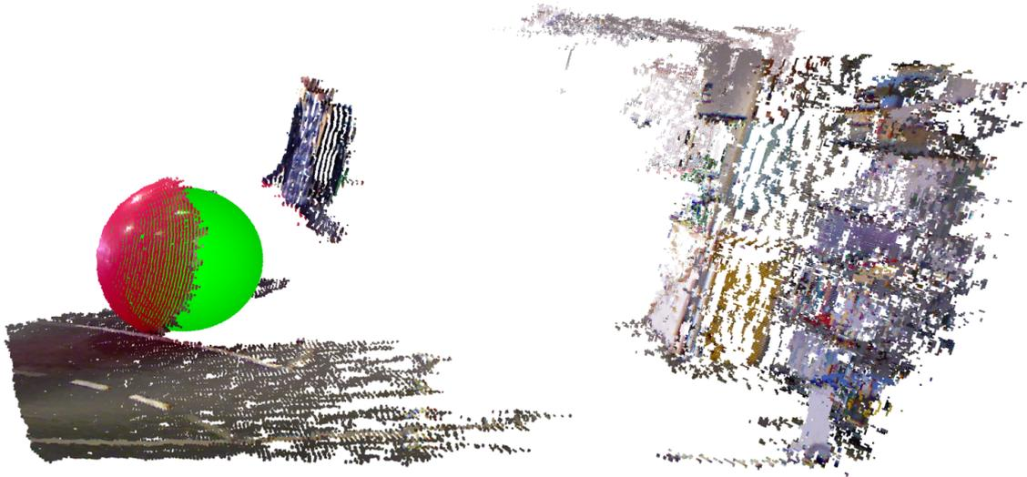
Figure 4.9: Ball detection (green sphere) in the point cloud acquired by the Microsoft Kinect 3D-depth sensor with RGB registration.
