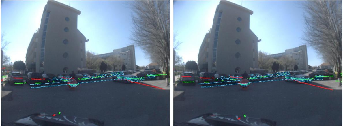
(a) Grid pattern calibration using 3D rigid body transformation.
