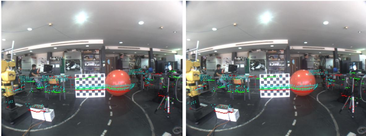
(a) Camera pose obtained through the 3D rigid body transformation method.
