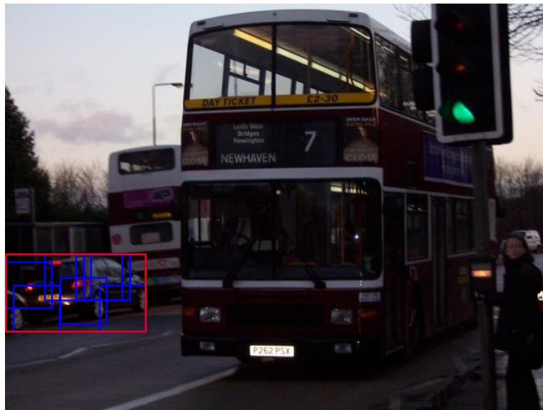
Figure 4: Example of a vehicle detection. The red box denotes the root filter detection while the blue boxes are part filters.
