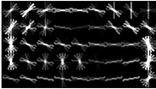
Figure 1: Asymmetrical root filter trained with warped positives and random negatives. This is just one of the root filters created for each class, in this case a car.
