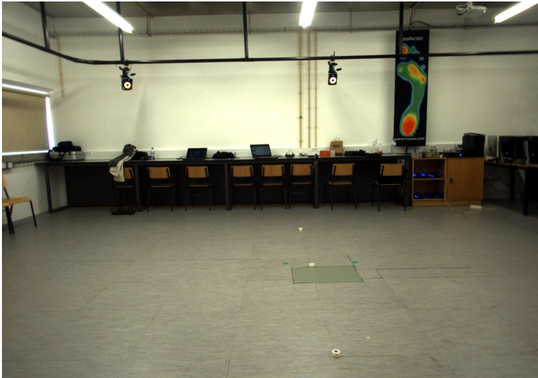
Figure 5.10: Motion capture laboratory. The laboratory contains a total of eight infrared cameras (only two are visible in the picture).
