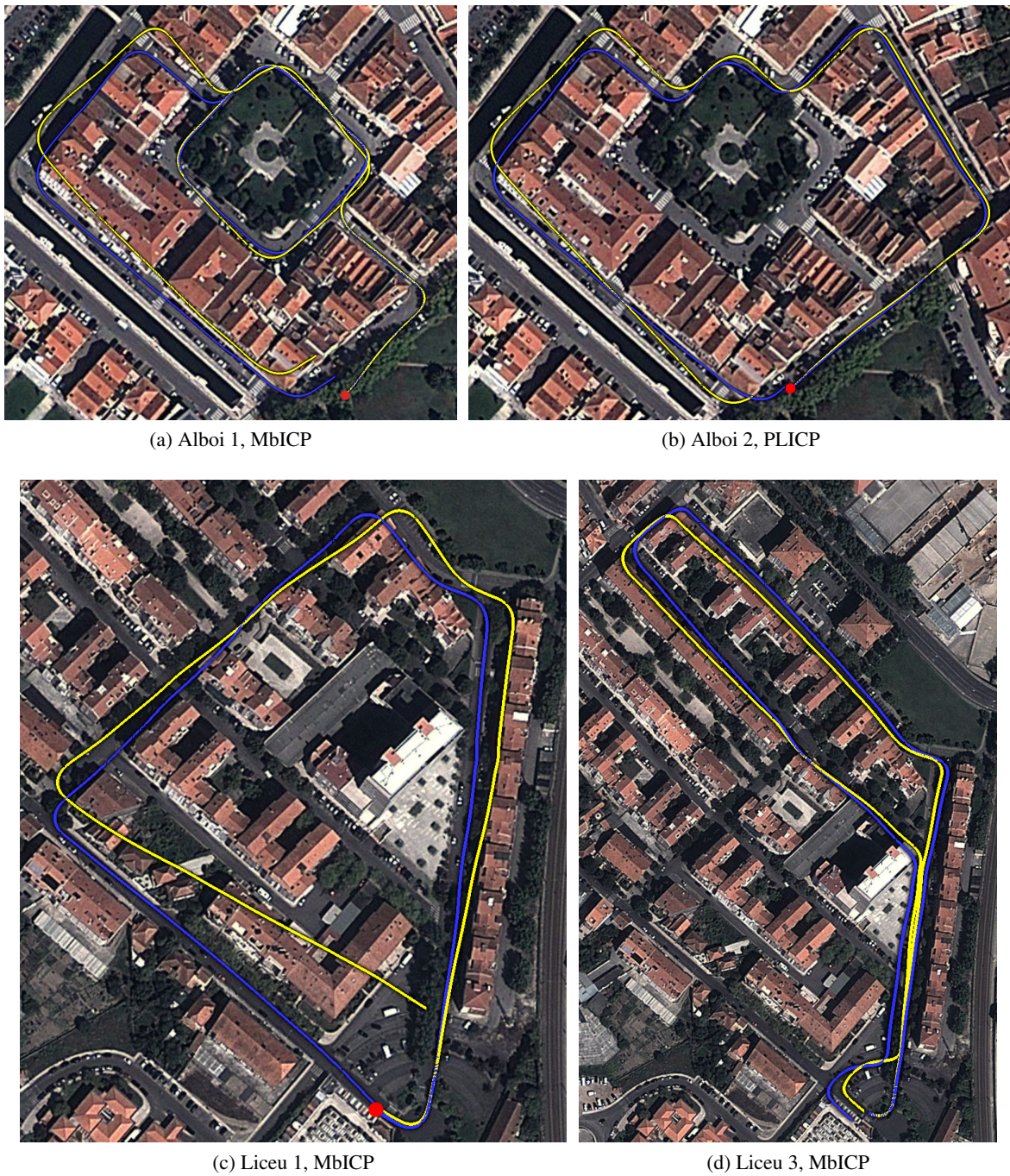
Figure 3.12: Several paths reconstructed using the proposed approach. The blue path corresponds to the path reconstructed using the odometry measurements while the yellow path corresponds to the proposed approach. The red dot indicated the start position of the trial. The error in the last corner of figure (c) was due to the local geometry of the road curve.
