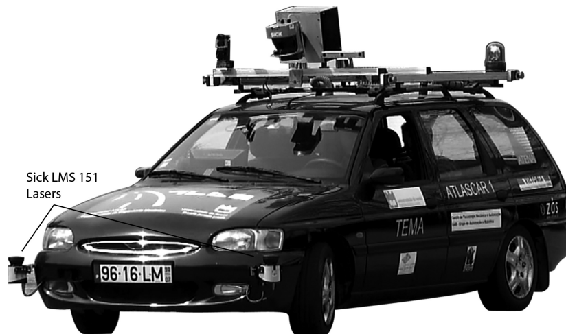
Figure 3.1: Picture of the Atlascar vehicle. In the proposed configuration the two Sick lasers have almost a complete coverage of the car's vicinity, having just a small blind spot in the rear of the vehicle.
